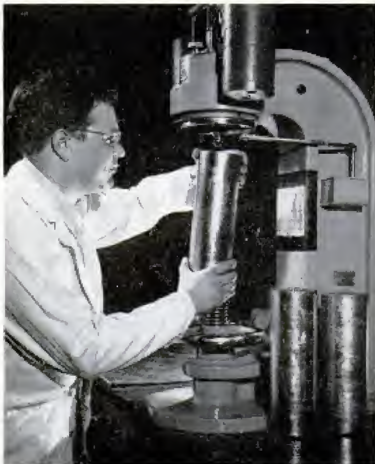
Glistening bars of zirconium, 99.9 percent pure, are raised from tank which has been flooded with water as a precaution against fire. Metal is deposited on wires by electrochemical action. Below, ingots of zirconium being tested for hardness before production use at Westinghouse Atomic Power Division
